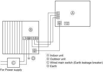
Perform wiring as shown in the diagram to the lower left. (Procure the cable locally) (Fig. 6-2)
