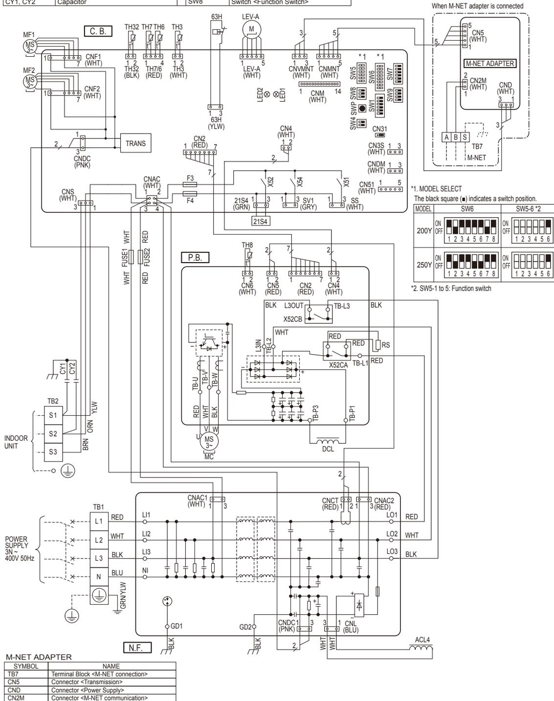
8-1. FIELD ELECTRICAL WIRING (power wiring specifications)
