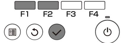
② With the **F1** or **F2** button, enter the refrigerant address, and press the
