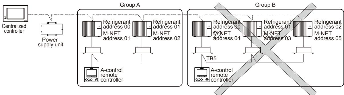
Note: In group B, M-NET address of the outdoor unit whose refrigerant address is "00" is not set to the minimum in the group. As "3" is right for this situation, the setting is wrong. Taking group A as a good sample, set the minimum M-NET address in the group for the outdoor unit whose refrigerant address is "00".
