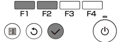
② With the **F1** or **F2** button, enter the refrigerant address, and press the
