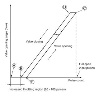
\* When the power is turned on, to register the valve position, a 2200 pulses valve close signal is output and is always set to point (A).
