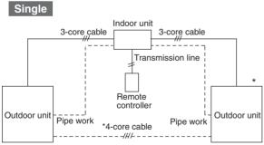
\* Two outdoor units connected when using PEH-P400-500MYA, therefore 4-core cable required in order to send and receive alternate defrost signal.
