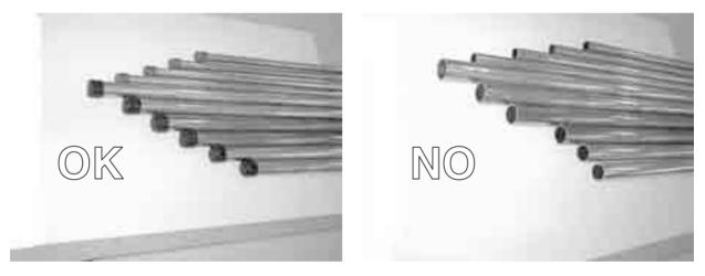
Both ends of the pipes should be sealed until immediately before brazing. Wrap elbows and T's in plastic bags for storage.
