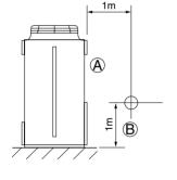
Sound pressure level in anechoic room 57 dB (A)
