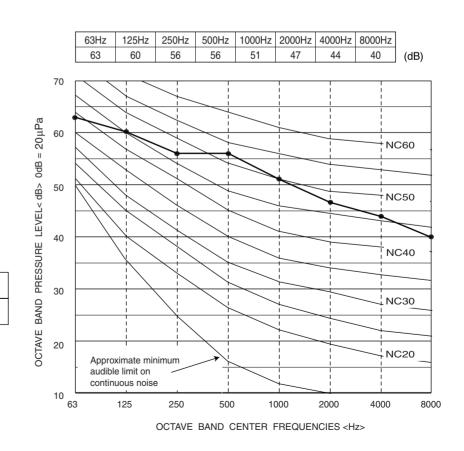
Note: The measuring point is 1m from the bottom of the unit (1m from the front of the unit).
