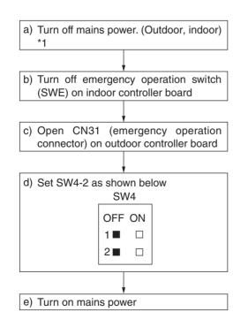
\* Before starting, recheck that the trouble allows emergency operation.
