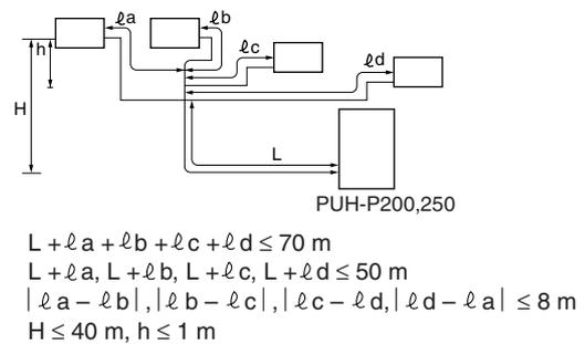
\* Total bends are 15 units, and max. bends are 8 units within  $L + l_a$ ,  $L + l_b$ ,  $L + l_c$  and  $L + l_d$ .
