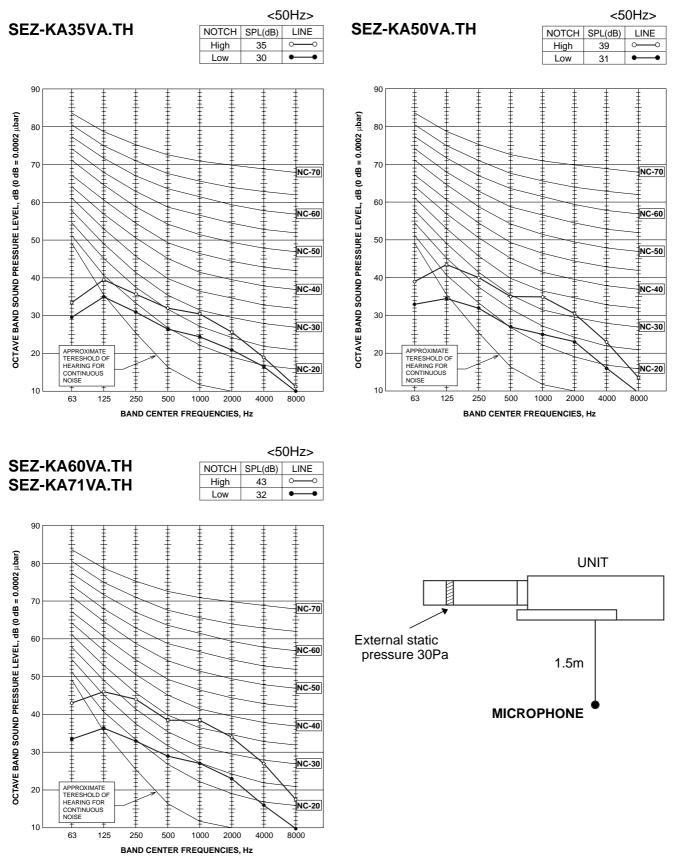
NOTE: The sound level is measured in an anechoic room where echoes are few, when compressor stops. The sound may be bigger than displayed level under actual installation condition by surrounding echoes. The sound level can be higher by about 2 dB than the displayed level during cooling and heating operation.
