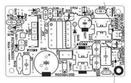
CNSK Connect to the indoor controller board (CNDK) between ① to ③ 220-240V AC
