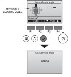
If all outlets are selected, \_\_\_\_ will be displayed the next time the unit goes into operation.
