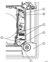
A Controller board CN4Y B Controller board CN6Y © 2 fasteners ④
