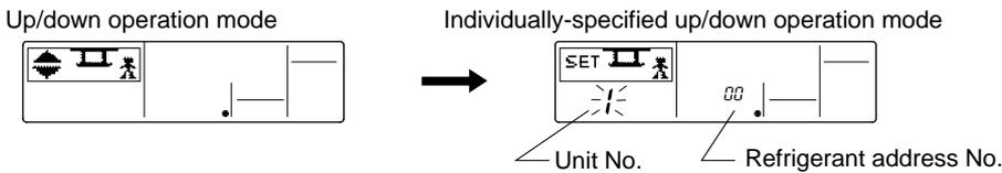
In the upper right figure, the air-conditioner for which the refrigerant address is "00" and the unit No. is "1" is currently selected.
