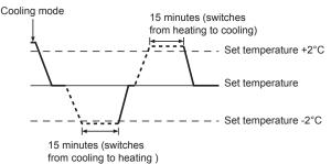
■ Because the room temperature is automatically adjusted in order to maintain a fixed effective temperature, cooling operation is performed a few degrees warmer and heating operation is performed a few degrees cooler than the set room temperature once the temperature is reached (automatic energy-saving operation).
