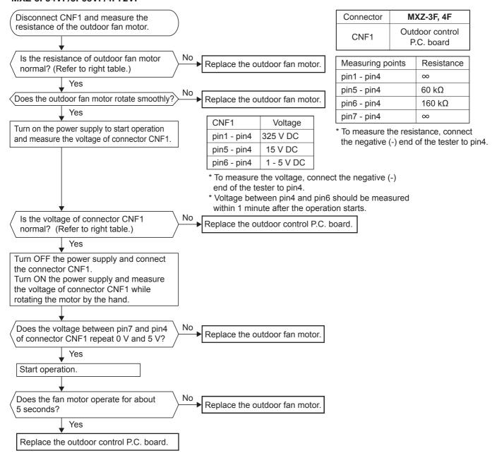
• When the operation frequency does not go up from the lowest frequency.
