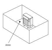
B) Install in a space with a depression height of 0.125 [m] or less.
