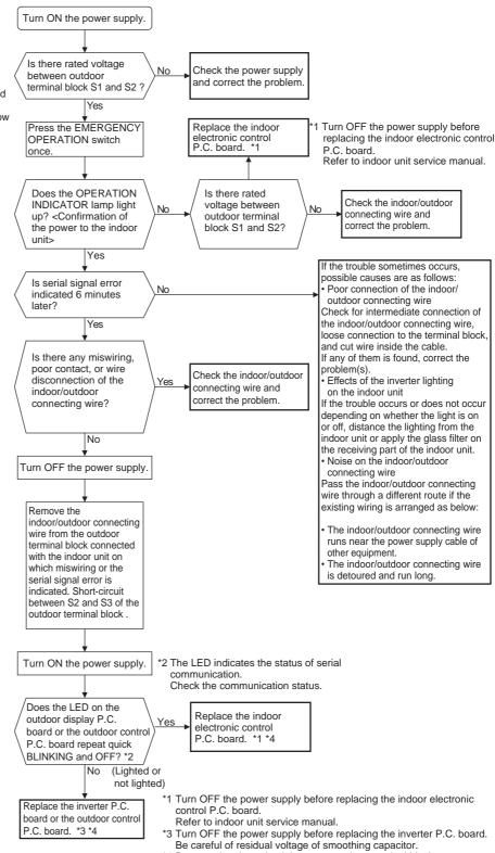
\*4 Remove the short-circuit between outdoor terminal block S2 and S3. Connect the indoor/outdoor connecting wire.
