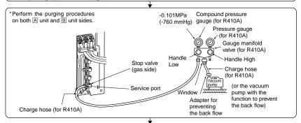
Remove the gauge manifold valve guickly from the service port of the stop valve.
