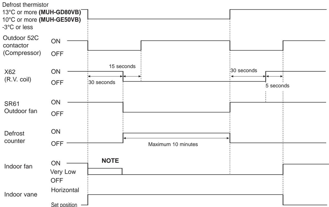
**NOTE:** • When the indoor coil thermistor reads above 18°C, indoor fan operates at Very Low for 30 seconds.
