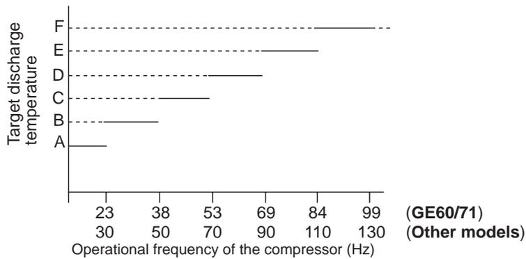
Reference value of target discharge temperature (COOL/HEAT °C)
