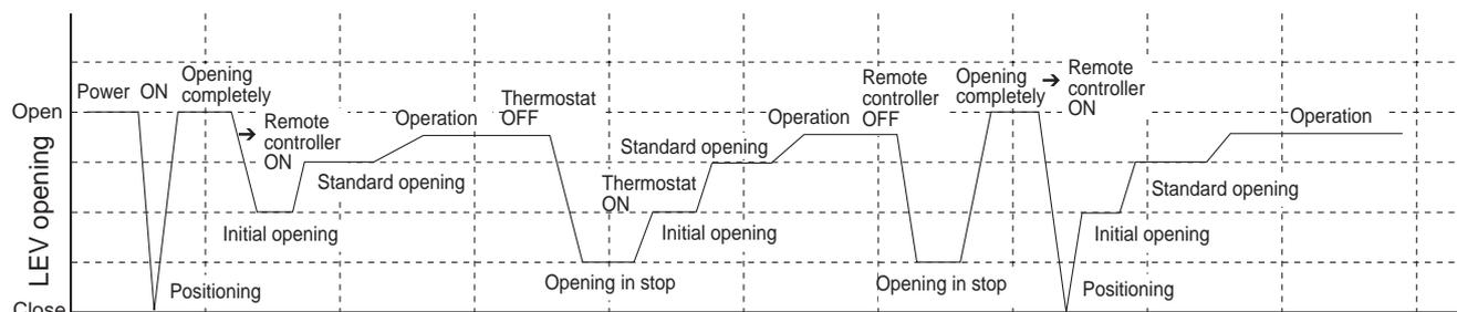
**NOTE:** Opening increases and decreases to be in the target discharge temperature during operation.
