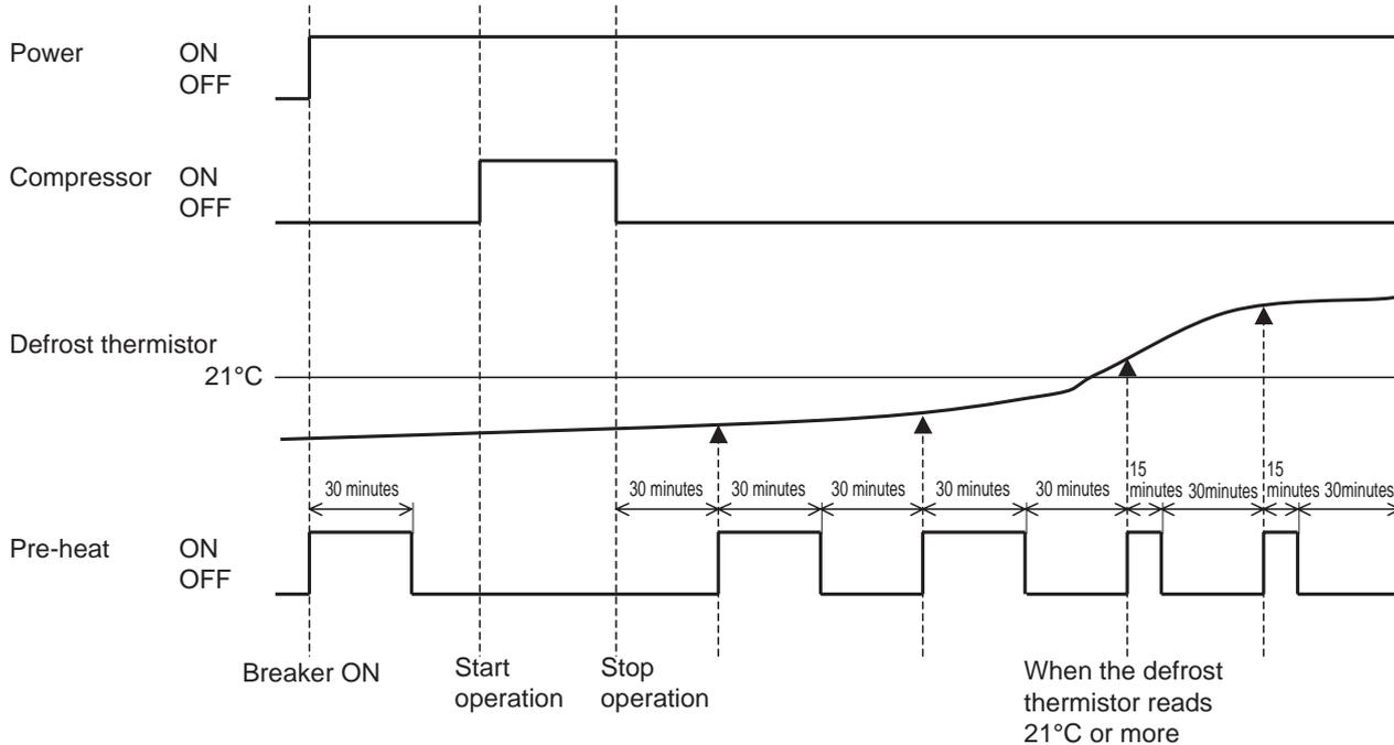
1. Pre-heat control is turned ON for 15 or 30 minutes\* after the breaker is turned ON.
