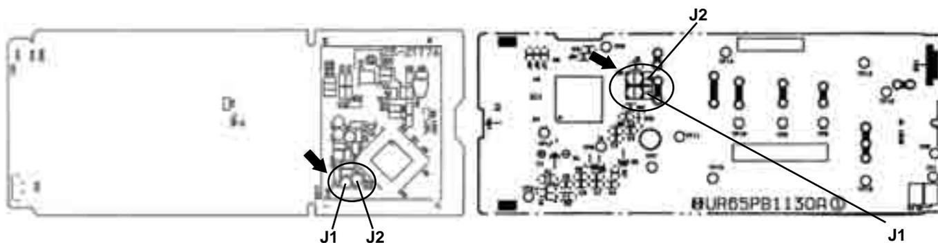
The P.C. board has the print "J1" and "J2". Solder "J1" and "J2" according to the number of indoor unit as shown in Table 1. After modification, press the RESET button.
