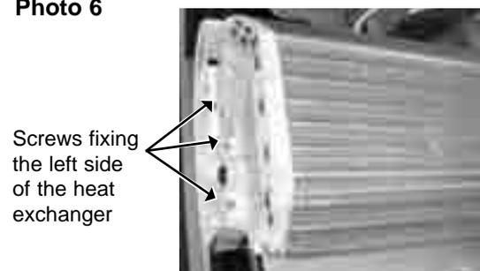
Screws fixing the left side of the heat exchanger
