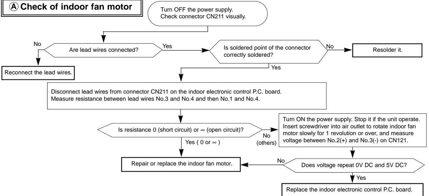
Indoor unit operates by pressing the EMERGENCY OPERATION switch, but doesn't operate with the remote controller.
