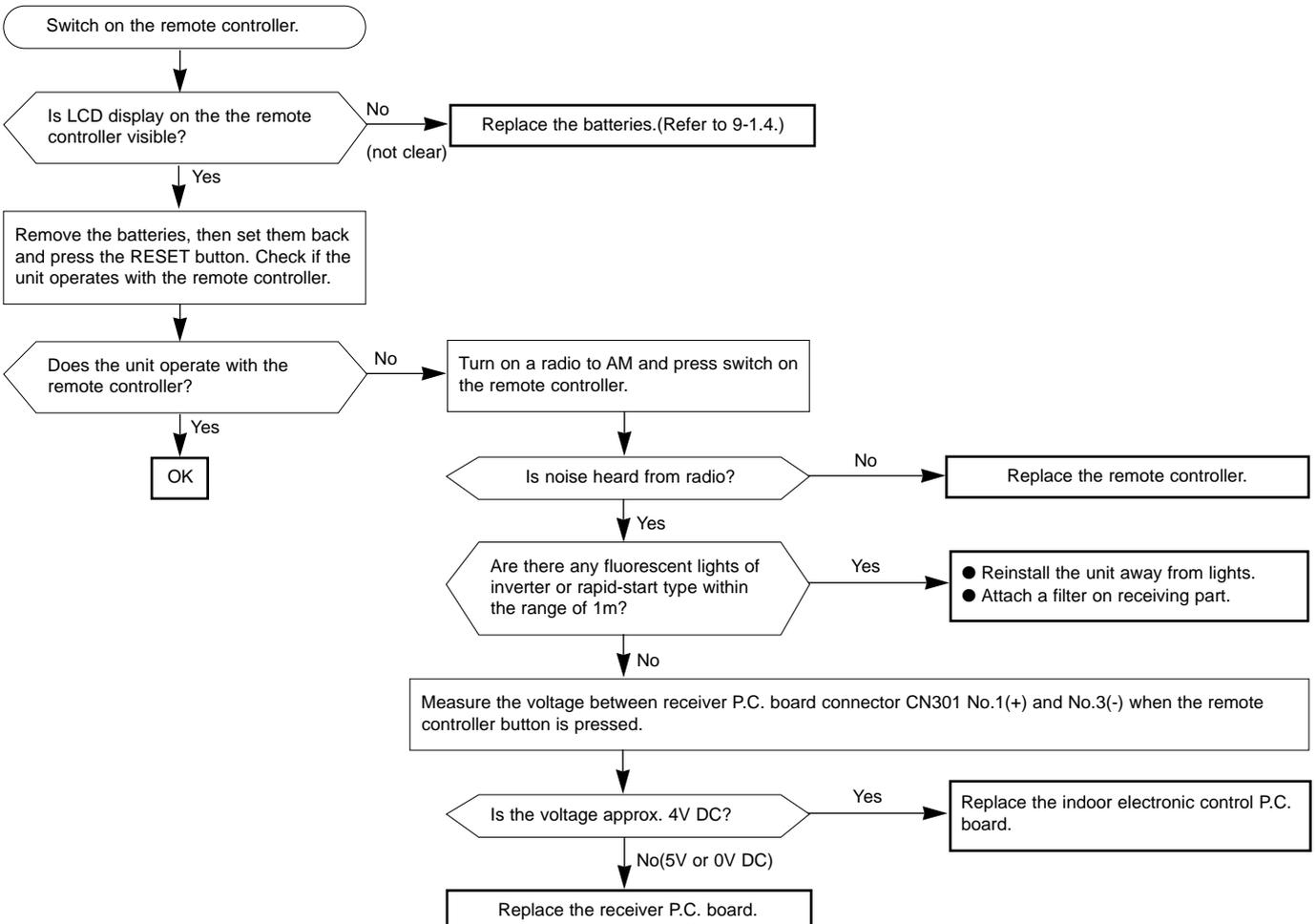
The unit doesn't operate with the remote controller. Also, the OPERATION INDICATOR lamp doesn't light up by pressing the EMERGENCY OPERATION switch.
