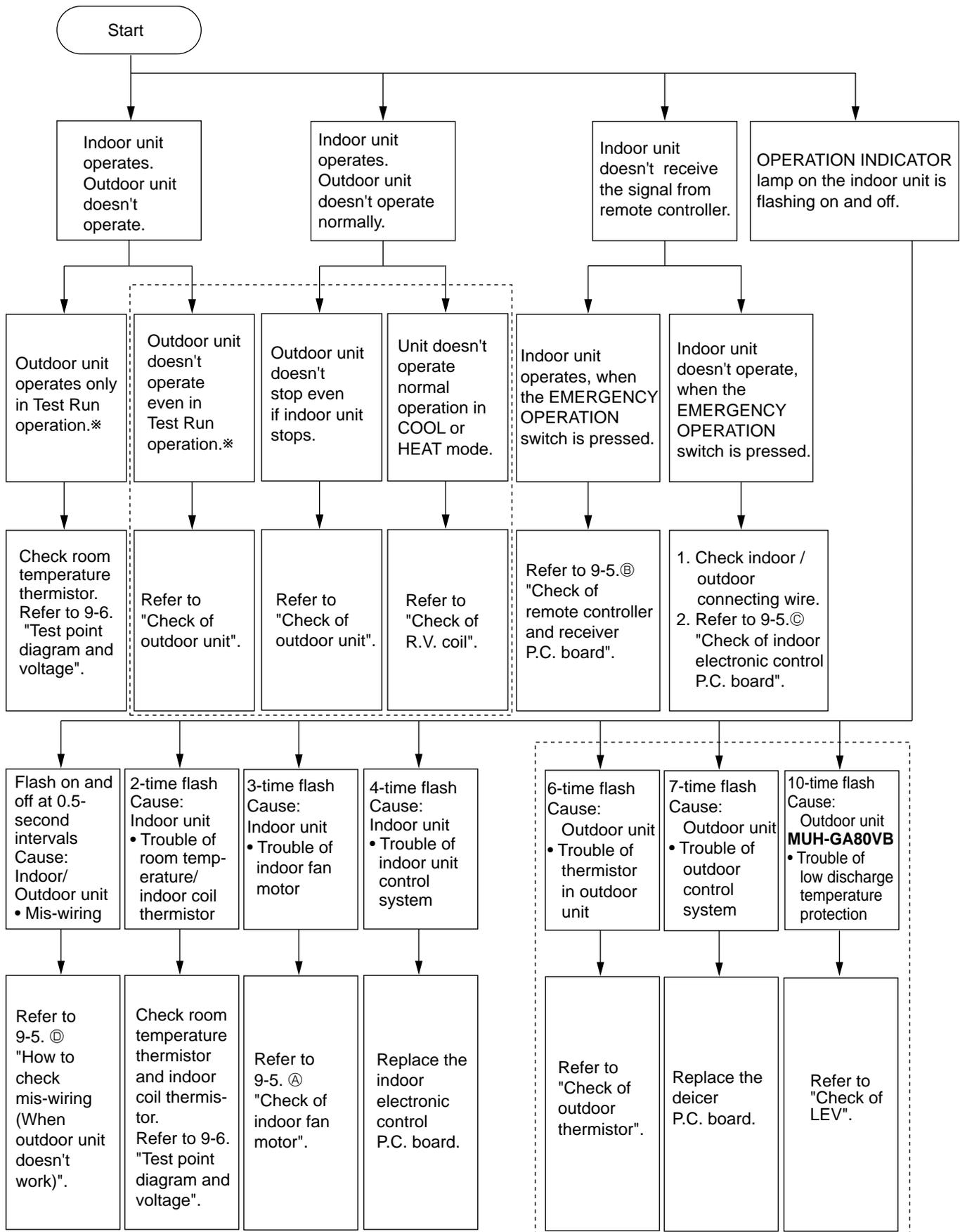
\*"Test Run operation" means the operation within 30 minutes after EMERGENCY OPERATION switch is pressed.
