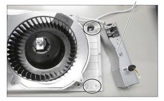
[2] Unscrew the screw (one PT screw 4x8, indicated by O), and remove the PCB cover.
