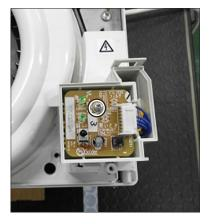
[3] Disconnect the connector from the display circuit board, and remove the circuit board (VL-36S).
