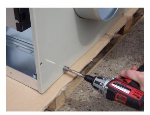
Align the back panel 7 to the Lossnay unit and fit using 3 x M6 X 12 set screws (12)
