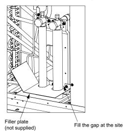
The gaps around the edges of through holes for pipes and wires on the unit allow water or mice to enter the unit and damage its parts. Close these gaps with filler plates.
