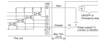
Use relays X1, X2, Y1, and Y2 that meet the following specifications. Contact rating Rated voltage >= 12VDC Rated current >= 0.1A Minimum applicable load =< 1mA at DC
