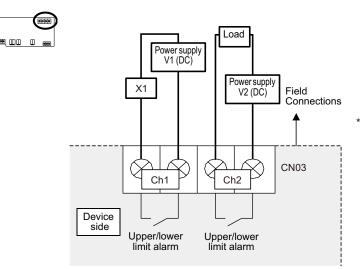
\* The contact of the internal relay is always ON during detection of an upper/lower limit alarm. (Level output)
