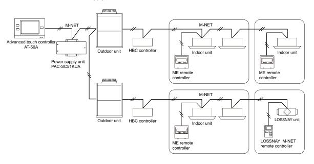
Fig. 1 Basic structure of AT-50A and PAC-SC51KUA
