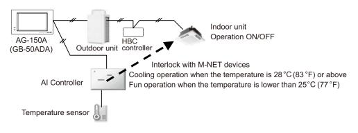
Interlock control of AI controller (example)
