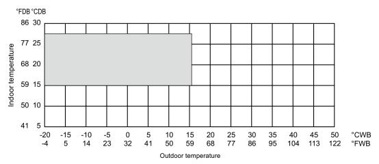
• Combination of cooling/heating operation (Cooling main or Heating main)
