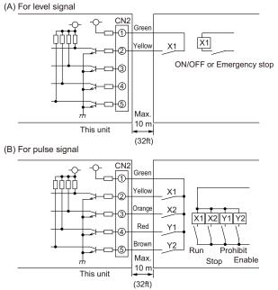
① The relays and extension cables, etc. must be prepared separately at the site.
