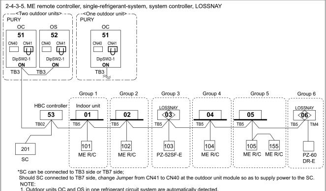
Outdoor units OC and OS in one refrigerant circuit system are automatically detected.
