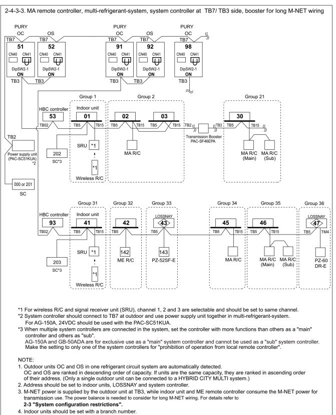
5. When a PAR-31MAA is connected to a group, no other MA remote controllers can be connected to the same group.
