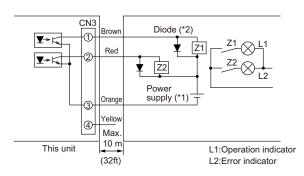
① " ON" signal and " Malfunction" signal will both be output.
