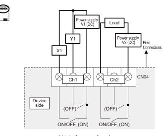
Operate (ON) output : Contacts closed Stop (OFF) output : Contacts open \*Upon pulse output, the (ON), (OFF) contacts close according to the output content. ((ON) and (OFF) refer to the junctions in the diagram.)
