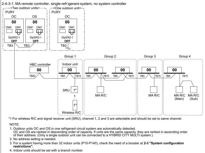
5. When a PAR-31MAA is connected to a group, no other MA remote controllers can be connected to the same group.
