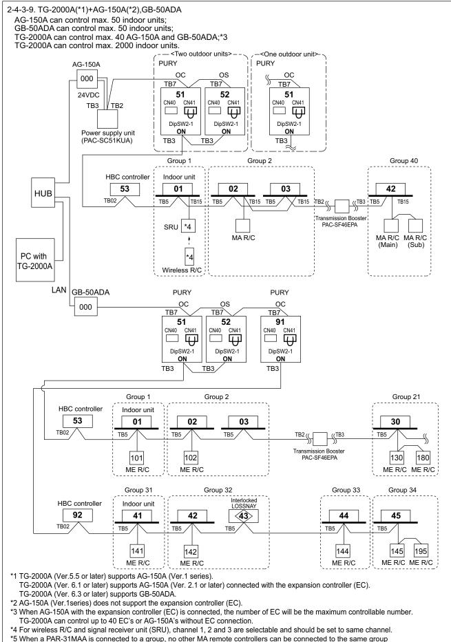
\*6 Only a single outdoor unit can be connected to a HYBRID CITY MULTI system.
