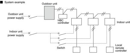
Restart of the HYBRID CITY MULTI needs to be careful. When no power supply to the outdoor unit, no power supply to the compressor case heater too. The compressor needed to be warmed up before running. When using above functions, power supply to the outdoor unit should be ensured.
