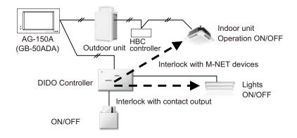
Interlock control of DIDO controller (example)
