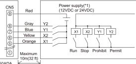
Use relays that meet the following specifications for X1, X2, Y1, and Y2. Contact rating  $% \label{eq:contact}$
