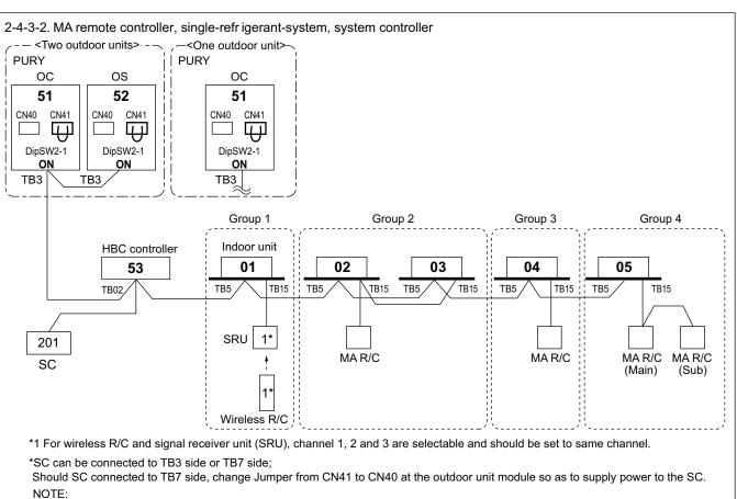
1. Outdoor units OC and OS in one refrigerant circuit system are automatically detected.
