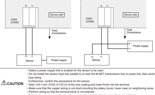
If strained, use a wire guide or junction terminal to alleviate the stress on the terminal block.
