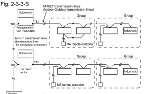
System controller A maximum of 6 System controllers can be connected to TB7
