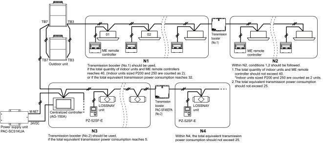
\*The figure above shows a system to which two outdoor units are connected, but only a single outdoor unit can be connected to a HYBRID CITY MULTI system.
