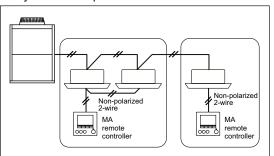
\*When a PAR-31MAA is connected to a group, no other MA remote controllers can be connected to the same group.
