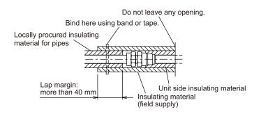
• Insulation materials for the pipes to be added on site must meet the following specifications:
