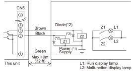
The "ON" signal is output even while the "Malfunction" signal is being output.
