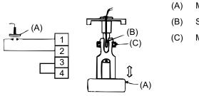
(A) Moving part(B) Switch(C) Magnet
