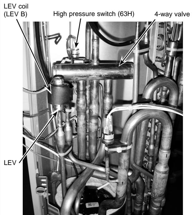
**Note 1:** Recover refrigerant without spreading it in the air.
