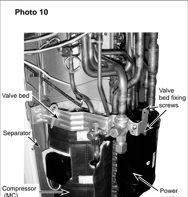
**13. Removing the power receiver**
