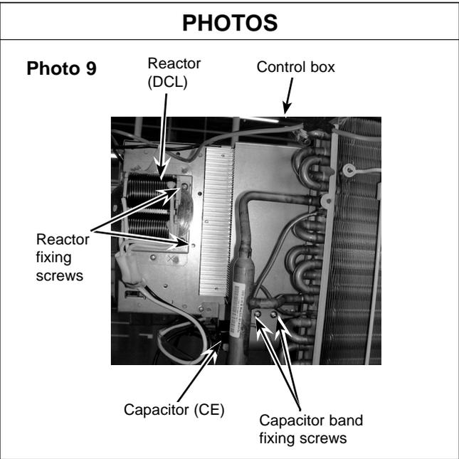
**12. Removing the compressor (MC)**
