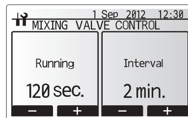
Mixing valve setting screen
