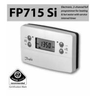
Before beginning programming, you should reset the unit. Open the flap on the front of the clock. Press the RESET button using a non-metallic object (e.g. end of a bic biro pen top). This will clear all previous pre-set programmes. (Fig. 1)
