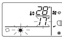
While the heating preset temperature display blinks, pressing the **TEMP. ▲** button increases the heating preset temperature, and pressing the **TEMP. ▼** button decreases the heating preset temperature.
