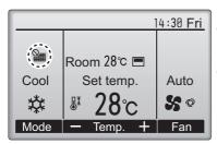
When the is displayed on the Main display in the Full mode, the system is centrally controlled and the filter sign cannot be reset.
