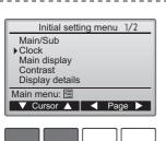
Move the cursor to the "Clock" with the F1 or F2 button, and press the SELECT button.
