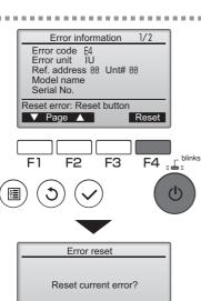
Press the F4 button or the ON/OFF button to reset the error that is occurring.
