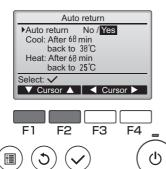
The screen to make the settings for the automatic return to the preset temperature will appear.
