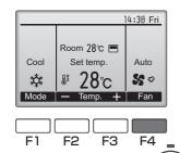
Press the F4 button to go through the fan speeds in the following order.
