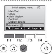
Move the cursor to the "Main display" with the F1 or F2 button, and press the SELECT button.
