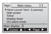
The following settings cannot be made from the sub remote controller. Make these settings from the main remote controller. "Main" is displayed in the title of the Main menu on the main remote controller.
