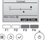
Adjust the contrast with the F3 or F4 button, and press the MENU or RETURN button.
