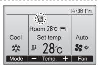
will appear on the Main display in the Full mode when the weekly timer setting for the current day exists.
