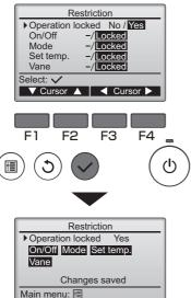
The screen to make the settings for the operation lock function will appear.
