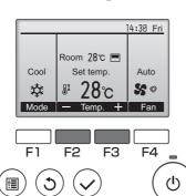
Press the F2 button to decrease the preset temperature by 1°C (1°F), and press the F3 button to increase.
