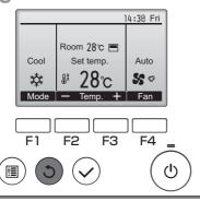
Press the RETURN button to exit the Main menu and return to the Main display.
