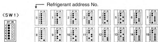
Factory setting: All switches are set to OFF (i.e., refrigerant address "0").
