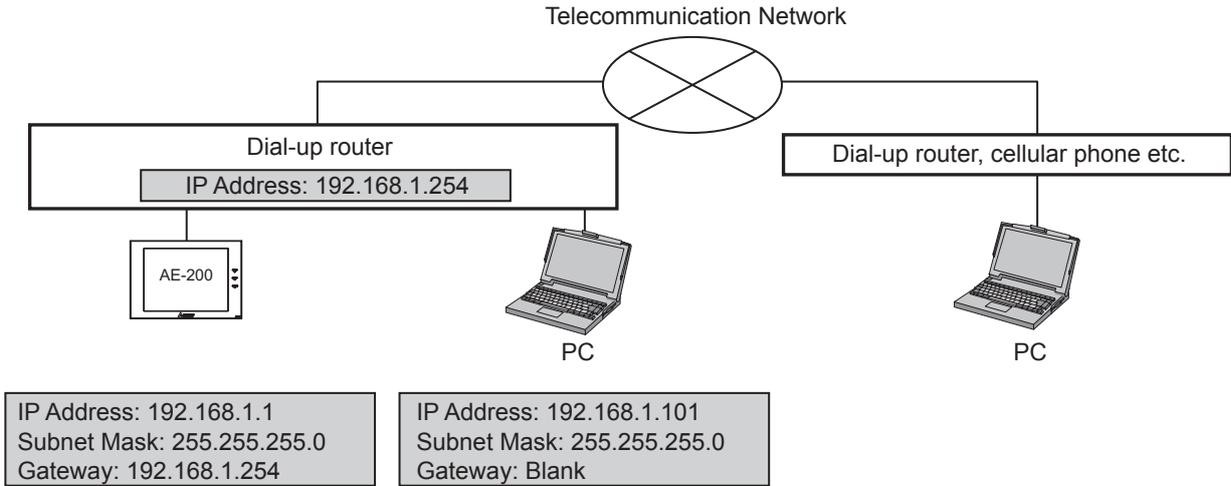
Note: [192.168.1.254] is recommended for use as the IP address of the dial-up router. Refer to the dial-up router instruction manual for details of how to set the IP address.
