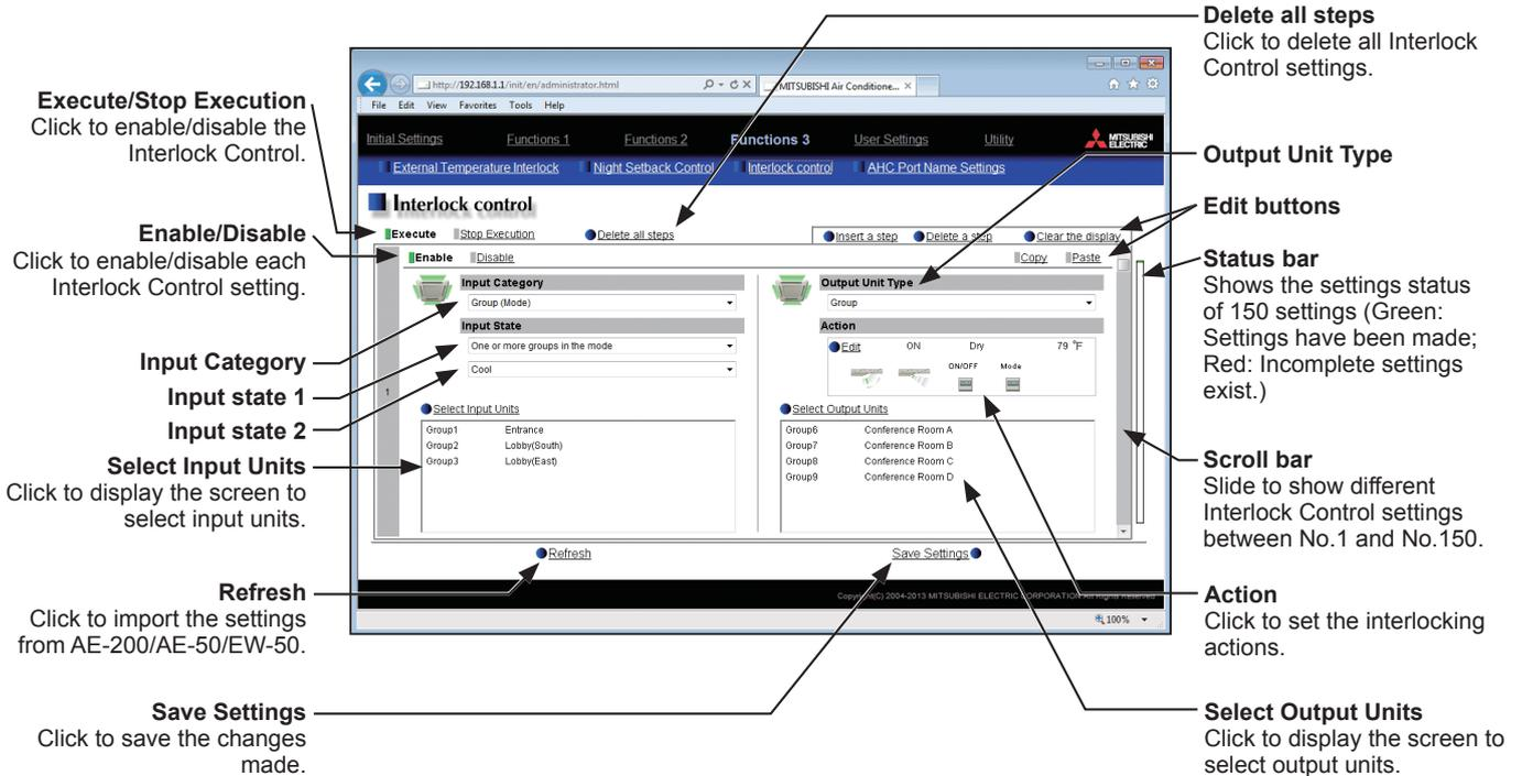
Up to 150 Interlock Control settings from No.1 through No.150 can be set for each AE-200/AE-50/EW-50. (Up to 600 Interlock Control settings can be made when one AE-200 and three or four AE-50/EW-50 controllers are connected.) The Interlock Control verifies the state changes in an ascending order of No.1 to No.150 every three to five seconds. When the interlocking conditions are met, the interlocking action commands will be issued to the output units.
