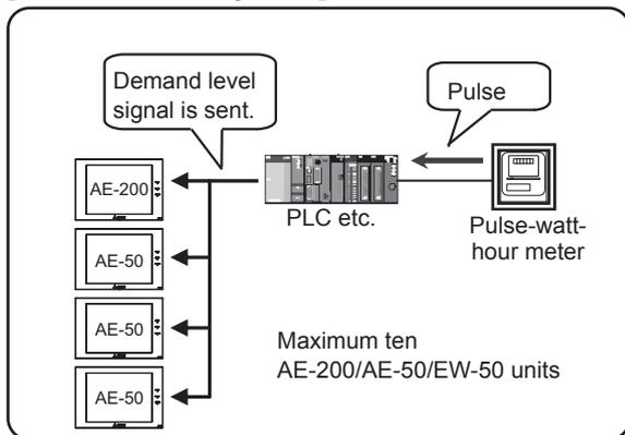
**(A) When the Peak Cut method [Demand-Input PLC] is selected**
