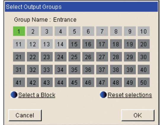
Note: If the Output Unit Type is set to [Group], air conditioning unit groups, LOSSNAY unit groups, Air To Water (PWFY) unit groups, HWHP (CAHV, CRHV) unit groups, and general equipment (connected via DIDO controller PAC-YG66DCA) groups are available for selection.
