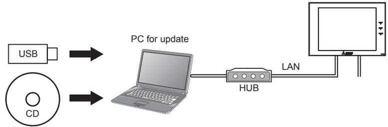
This manual explains how to update the software using a Web browser ( ② ). For how to update the software by directly reading the update file in a USB memory device ( ① ), refer to the AE-200 Instruction Book or Installation Manual.
