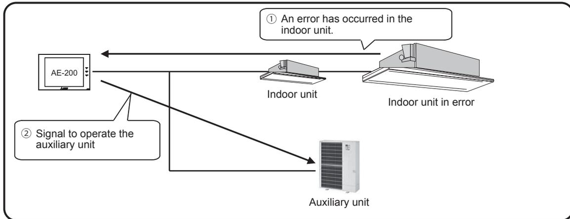
Example 7: Interlocked operation of the indoor units
