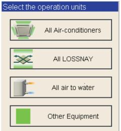
(2) After you have made the settings on the screen for batch operation, click [OK] and only the items for which operation was performed will be sent to all the air conditioner, ventilator (LOSSNAY) groups, Air To Water (PWFY) groups or general equipment groups.
