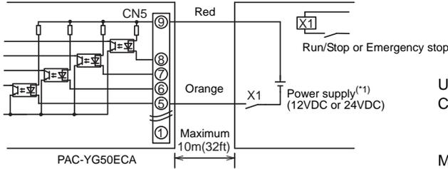
Use relays that meet the following specifications for X1, X2, Y1, and Y2.
