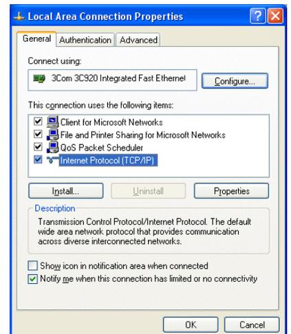
(4) In the [Internet Protocol (TCP/IP) Properties] dialog, click [Use the following IP address] and enter the IP address (for example, “192.168.1.101”) that you want to set in the IP address field.
