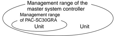
When using a system where PAC-SC30GRA is controlled by a different system controller. PAC-SC30GRA is set as the slave system controller. In this case, the group settings are not performed with PAC-SC30GRA.
