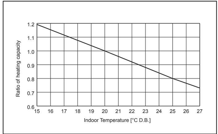
**Figure 10 Outdoor unit temperature correction**
