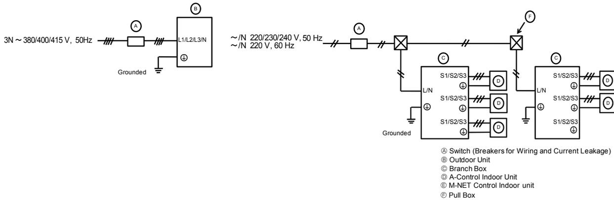
■ Schematic Drawing of Wiring : When using a Branch Box and M-NET control indoor unit (example)
