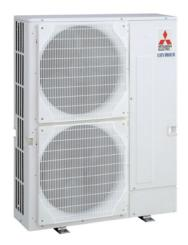
The latest in Mitsubishi Electric Y Series technology incorporated within the new City Multi 6hp model allows up to 12 indoor units to be connected to a single outdoor unit, using the standard branch/header pipework system proven in the larger models. Utilising the latest Mitsubishi Electric Inverter technology, the system is fully controllable with all City Multi controllers or linked to third party BEMS.
