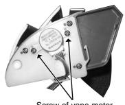
Screw of vane motor
