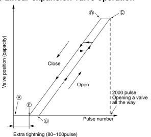
\*\* When the switch is turned on, 2200 pulse closing valve signal will be send till it goes to @ point in order to define the valve position.
