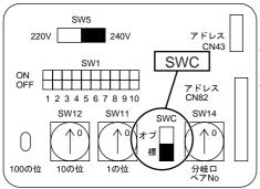
With this function, air comes out simultaneously from the upper and lower air outlets so that the room can be cooled or heated effectively. This function is set using the switch SWC on the address board.
