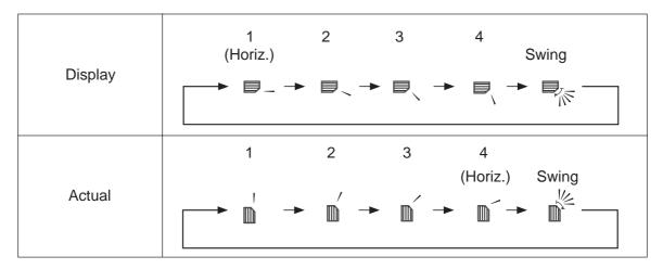
The airflow direction for the lower air outlet damper cannot be set. The airflow direction is automatically controlled by a computer.
