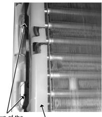
Screws of the heat exchanger Hai
