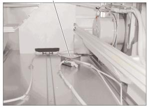
②Take the damper motor out of the cover.
